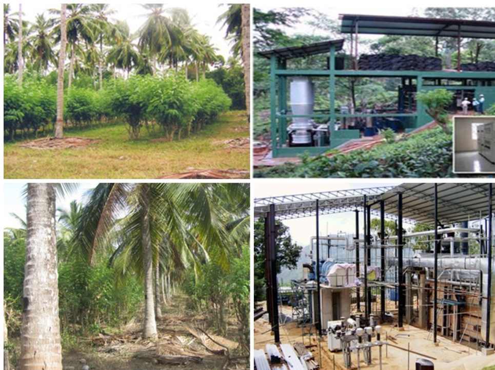
Figure 16.7 A. Gliricidia intercropped with coconut in Sri Lanka. The trees are pruned every eight months to provide the biomass feedstock for electrical power generation; B. a 290 kW gliricidia fueled power plant in Sri Lanka, C. D. A 1.5 MW gliricidia fueled power plant in Sri Lanka
