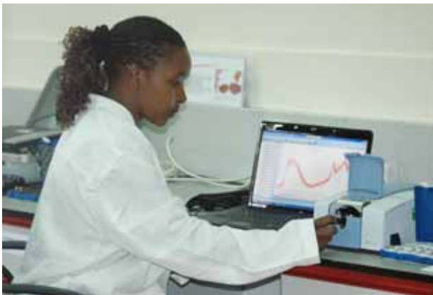
Figure 4.2 Portable mid-infrared spectrometer being used for rapid characterization of soil samples
