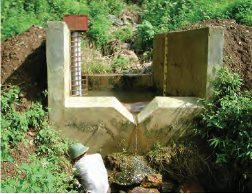
Fig. 2.3. Field measurements of erosion on a catchment scale (Carried out by the Managing Soil Erosion Consortium - MSEC Vietnam and IRD).
