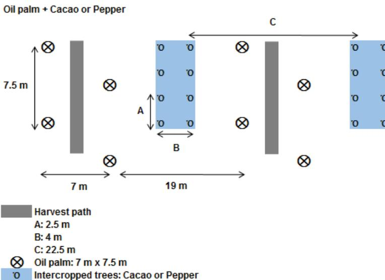
**Figure 6.3.** Design and spacing of intercropping oil palm with Cacao or Pepper
