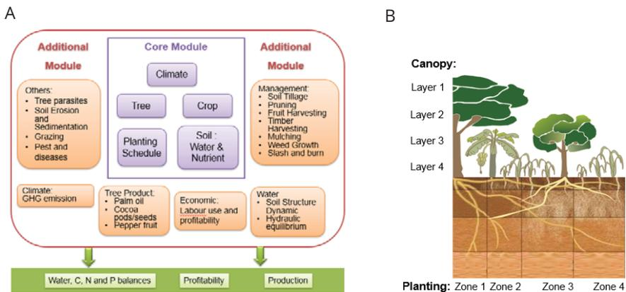
Figure 6.2. Main modules in WaNuLCAS model and its output (A), configuration of the models planting zones, canopy layers and soil layers (B)
