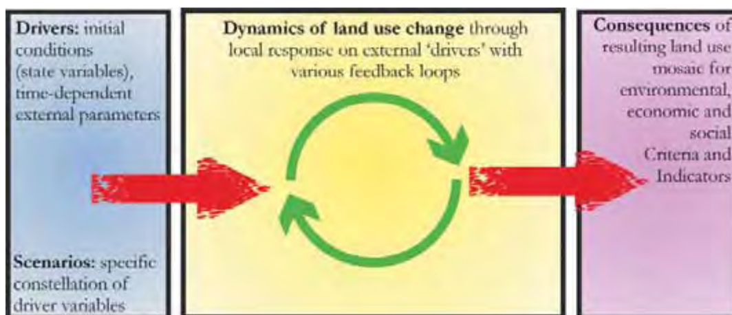
Figure 5.1. Generic structure of a model that translates 'driver' or exogenous variables to the time bound responses in a landscape, which has consequences ('externalities' in as far as they are not part of the feedback loops in the dynamic section) for criteria and indicators of system performance; scenarios refer to specific combinations of driver variables that represent changes in higher level systems.
