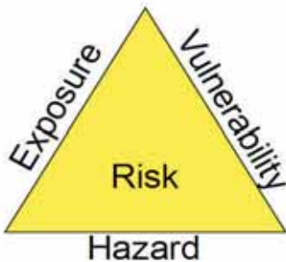
Figure B.2a. The risk triangle shows risk as the product of hazard × exposure × vulnerability. Source: Crichton (1999)
