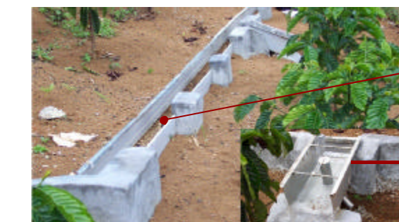
Runoff plot with gutter and 'Chino' meter for measuring soil loss and runoff
