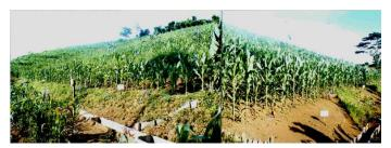
The natural vegetative buffer strips spacing experimental field in a 45 % slope located in MOSCAT Campus, Claveria, Misamis Oriental. This also features the erosion monitoring device, the tipping bucket method (sediment through and tipping bucket), to monitor eroded soils and run-off water, and the raingauge.
