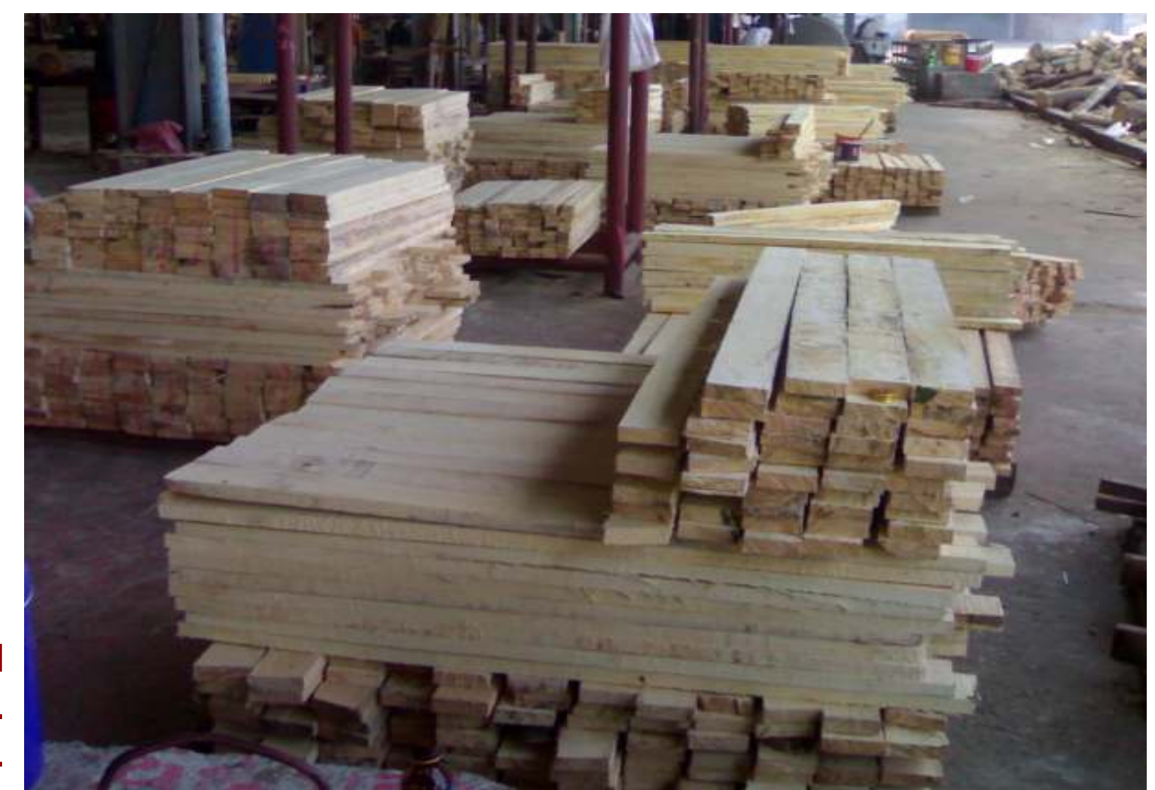
Planks of rubber timber prepared for chemical treatment. Photo: Adrián M.
