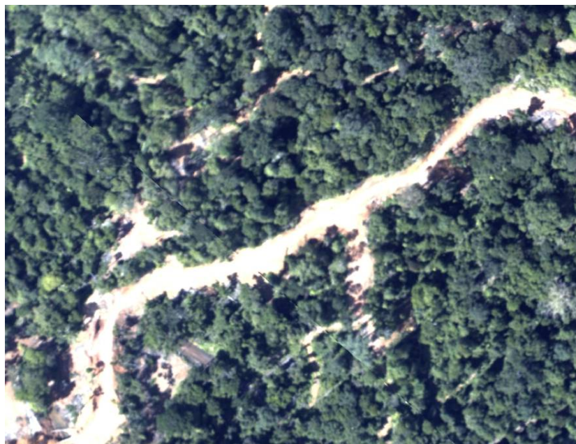
Figure 10 A logging road with skid trails emerging from it.
