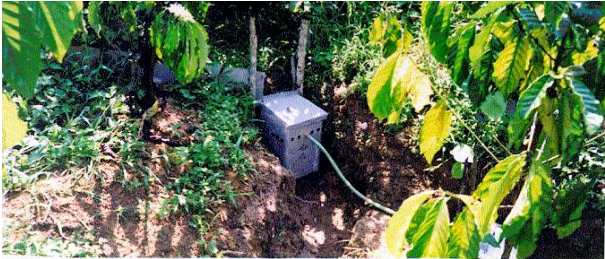
Figure 3. Sediment Collector to Measure Sediment Inflow
