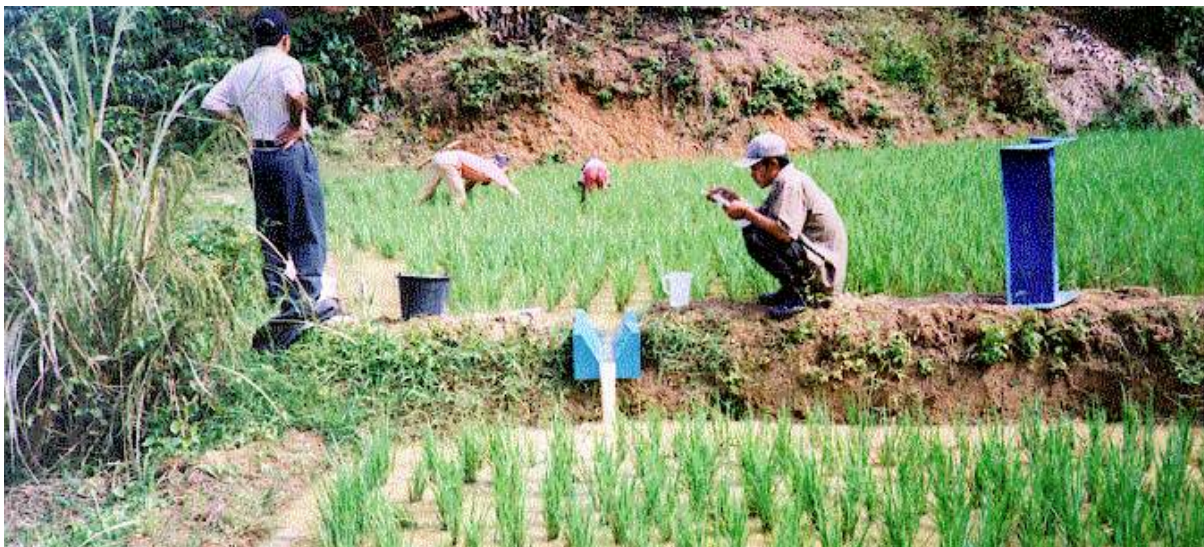
Figure 2. Measurement of Sediment Concentration Using Parshall Flume
