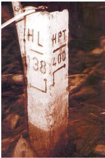
Boundary marker in the field of two classes of forest: HL = protection forest, HPT = limited production forest
